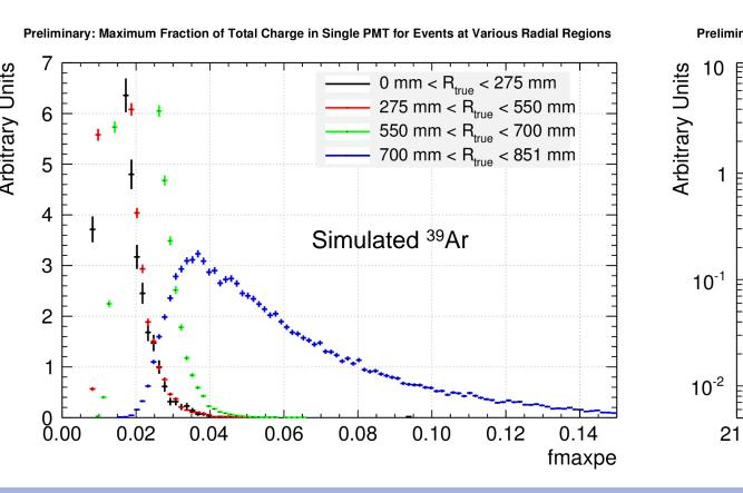
"fmaxpe" - The fraction of light detected by the PMT that detects the largest amount of charge "nhit" - The number of PMTs that record pulses during an event
