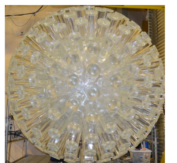
Acrylic vessel, after bonding of the LGs
