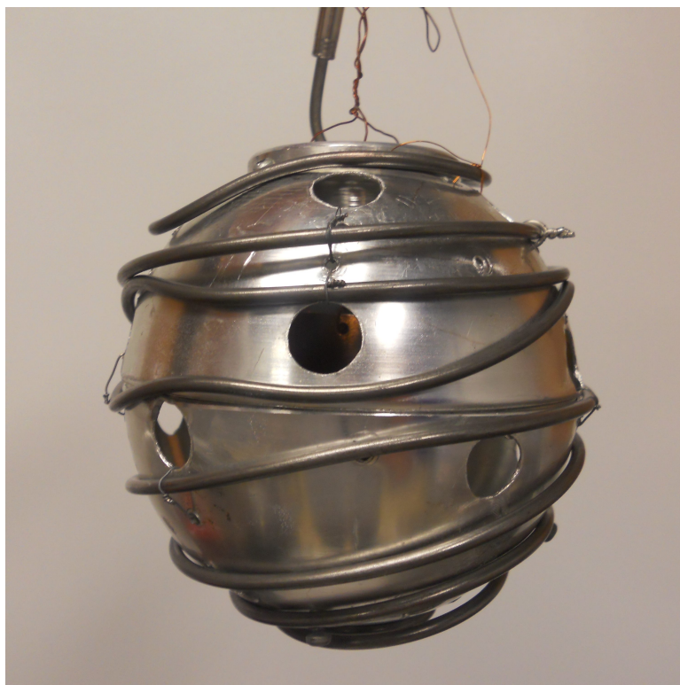
Figure 3.1: 11 cm in diameter prototype aluminum TPB source with Watlow heating wire wrapping the outside.
