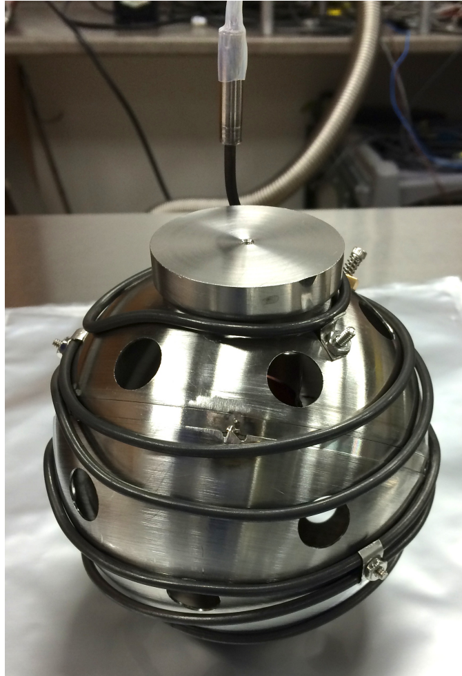
Figure 3.3: Final stainless steel TPB deposition source. The Nichrome wire is held in thermal contact with the stainless steel sphere by compressed stainless tabs. A stainless top hat was machined from which the copper crucible was attached.
