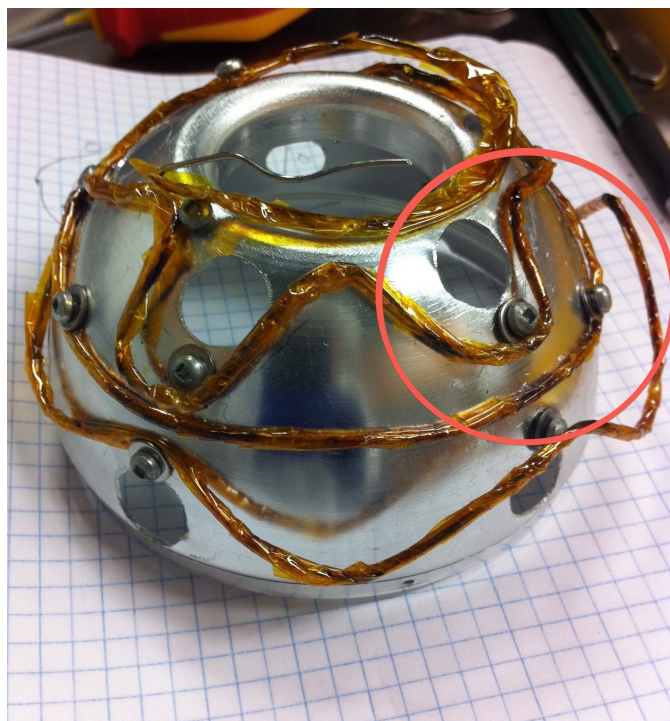
Figure 3.2: The prototype aluminum source with original Nichrome wire wrapped in Kapton tape for insulation. Charring, visible by the dark discoloration in the yellow Kapton tape, is highlighted by the red circle.
