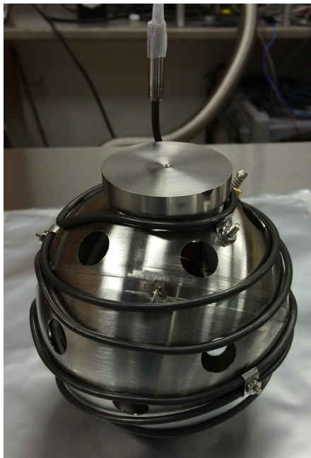
Figure 4. Final stainless steel TPB deposition source. The coil heater is held in thermal contact with the stainless steel sphere by compressed stainless tabs. A stainless steel top hat was machined from which the inner copper crucible is attached.
