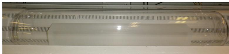
Figure 4.3: A 2 kg acrylic block is placed in the boat, and the boat is loaded before the vaporization furnace is turned on.
