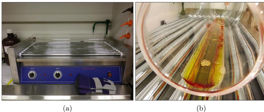
Figure 4.6: The residue from vaporization is removed from the boat by rinsing with aqua regia. (a) The boat rotates and is heated. (b) Aqua regia is poured into the boat and reacts for 1 h before being collected. The aqua regia rinse is repeated, and finally there is a quick rinse with UPW.
