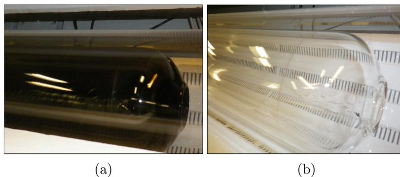
Figure 4.5: Acrylic vaporization produces too much char to manage during rinsing and counting. (a) The entire boat is covered and becomes opaque from 2 kg of the RPT acrylic used for the DEAP-3600 AV. (b) After vaporization, air is added to the vaporization furnace to remove the char.
