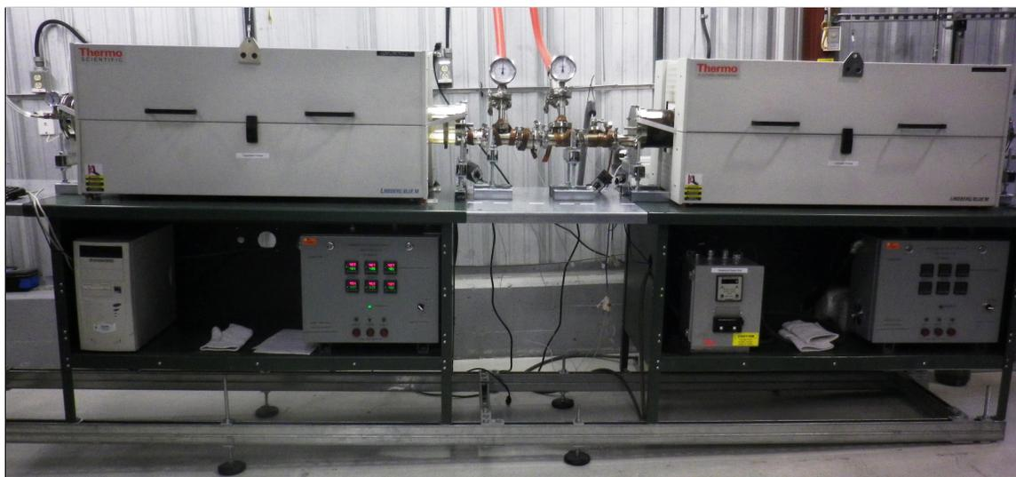
Figure 4.1: The acrylic vaporization system is on surface at SNOLAB. Acrylic is vaporized in the furnace on the left, and the MMA vapour is incinerated in the furnace on the right [56].
