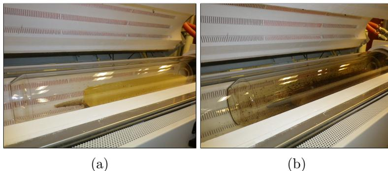
Figure 4.4: The DEAP-3600 AV acrylic from RPT turns yellow, drips, splatters, and produces black char. The block slides downstream due to an intentional incline. (a) 20 min and (b) 30 min after the start of vaporization.
