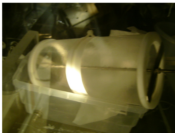
FIGURE 4. DEAP-1 acrylic insert with a solidified coating, after disassembling the spin coater.
