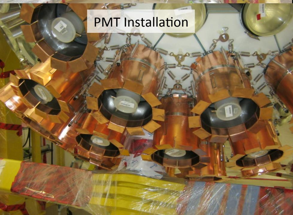
Installed LED fibre system reflector
