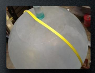
DEAP-3600 vessel constructed and delivered to University of Alberta (June 2012) for machining of light guide stubs
