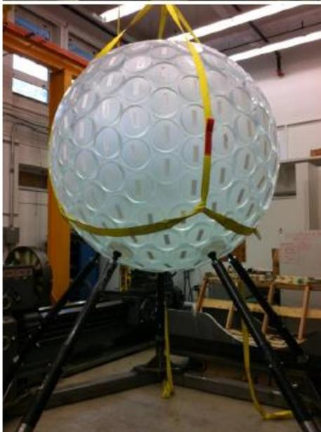
Bonded underground, finish machined and then light guides attached:
