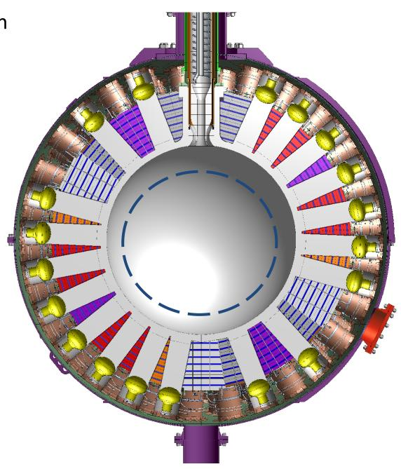
Cooling achieved with coils in neck fed with liquid nitrogen from and vapour return to a large dewar.
