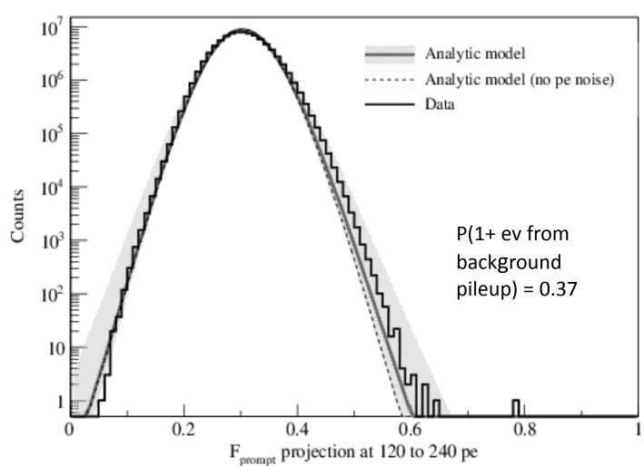
DEAP-1 PSD measurements agree with a model based on counting statistics and measured noise parameters. The model was applied to DEAP-3600 parameters.
