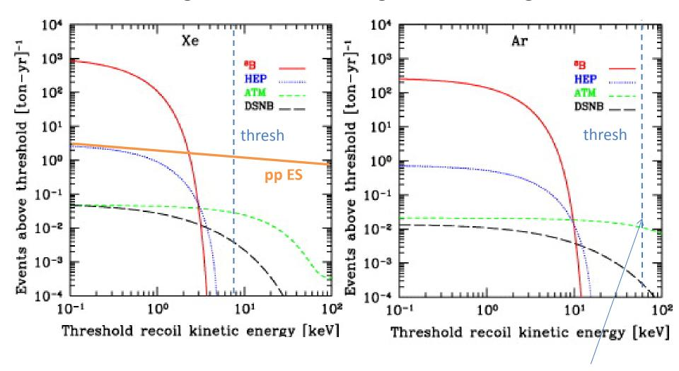
Target sensitivity for DEAP-50T (50 Tonne Fiducial Argon) is at ultimate limit of atmospheric neutrinos
